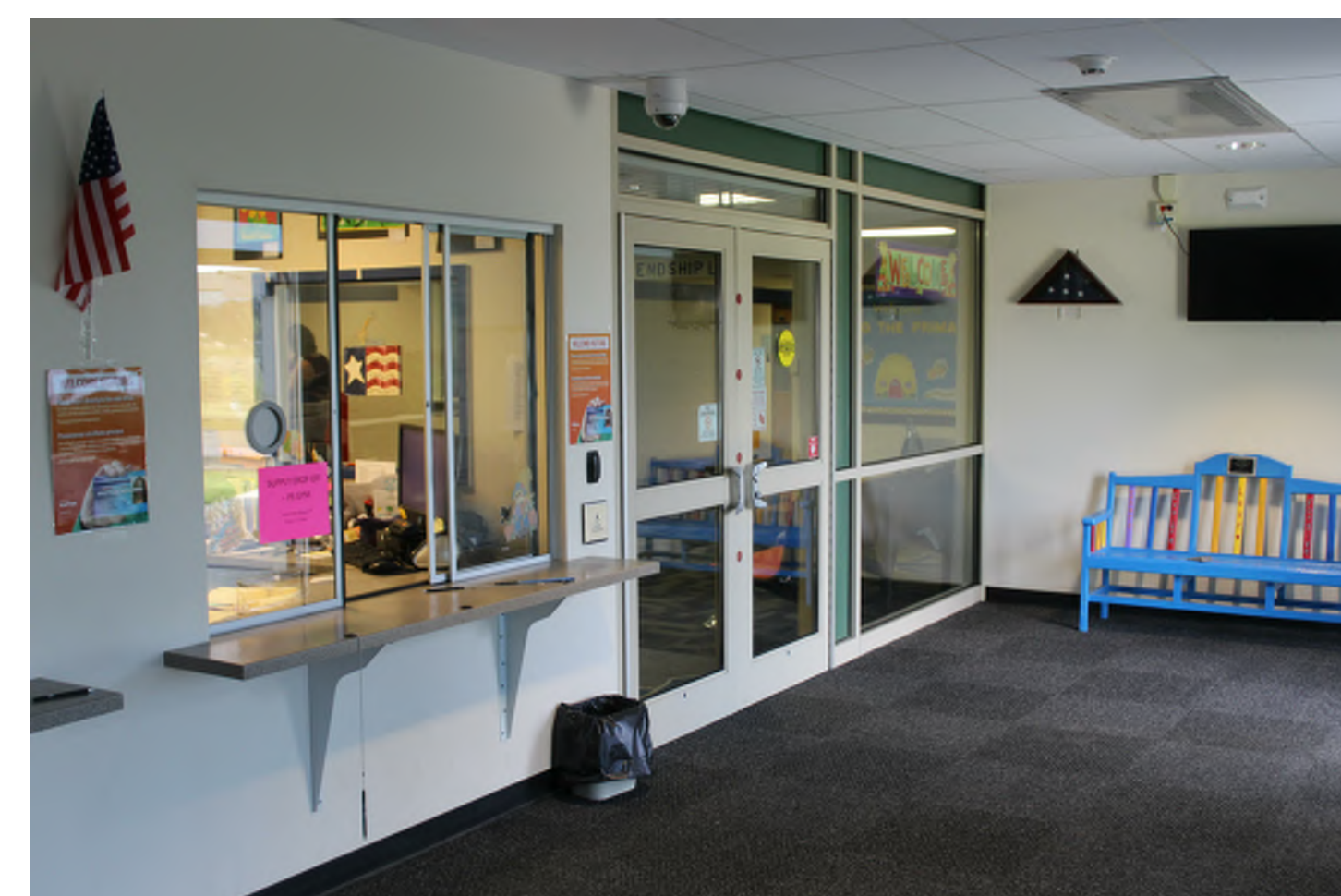
Primary School Vestibule Existing windows are open to intruders and easily compromised. Sliding windows would be replaced with fixed, bullet-resistant windows and surrounding doors/windows would receive impact-resistant film.
